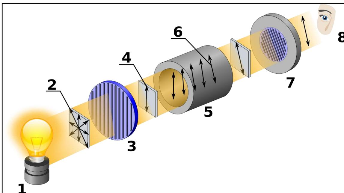
A polarimeter has a light source, a nicolprism to produce plane polarized light. This light passes through a solution in the sample holder. The light rotates and angle of rotation is observed from the other side.
